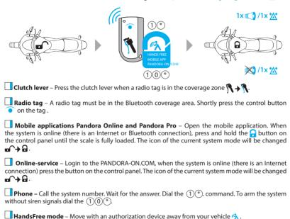
■ VALET button – Press and hold the VALET button for 3 seconds. The system will be armed in 30 seconds. The LED indicator is lighting red during the countdown
